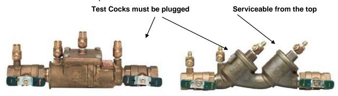
This new double check valve assembly must be installed at least one foot away from the water meter but as close as practical to the meter. The backflow prevention assembly must be certified by a Certified Backflow Technician after it is installed and prior to the Plumbing Inspection.
